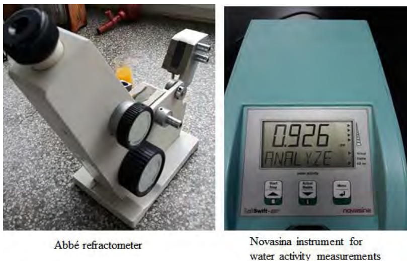
Figure 2. Abbé refractometer and Novasina instrument for water activity measurements
